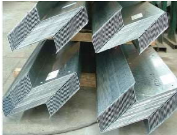
Figure 1 Cold-formed light-gauge steel members
