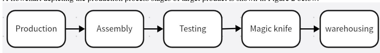
Figure 2 production processes of Li-ion Battery module of BYD
